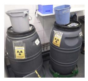
**Photo 7:** Liquid effluent barrels in the tritrium laboratory
